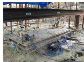
Bi-directional static load testing surrounded by Top-Down anchors
