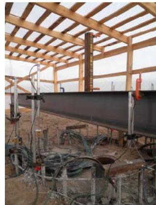
Pile head during bi-directional static load testing
